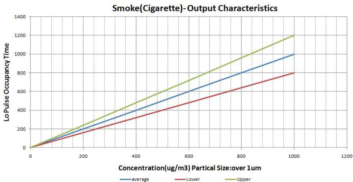
**Fig 3 Photoelectric linear**
