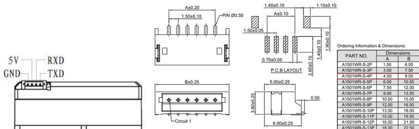
**Fig 2** Connector Dimensions
