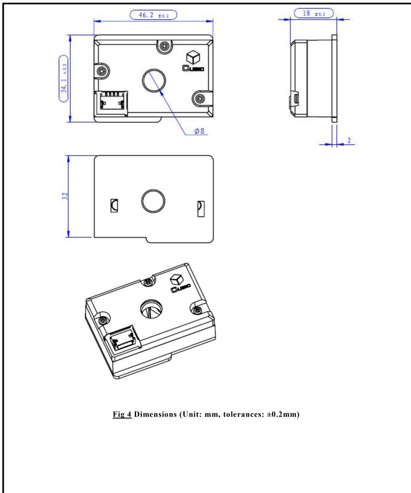
**Fig 4 Dimensions (Unit: mm, tolerances:  $\pm 0.2$ mm)**
