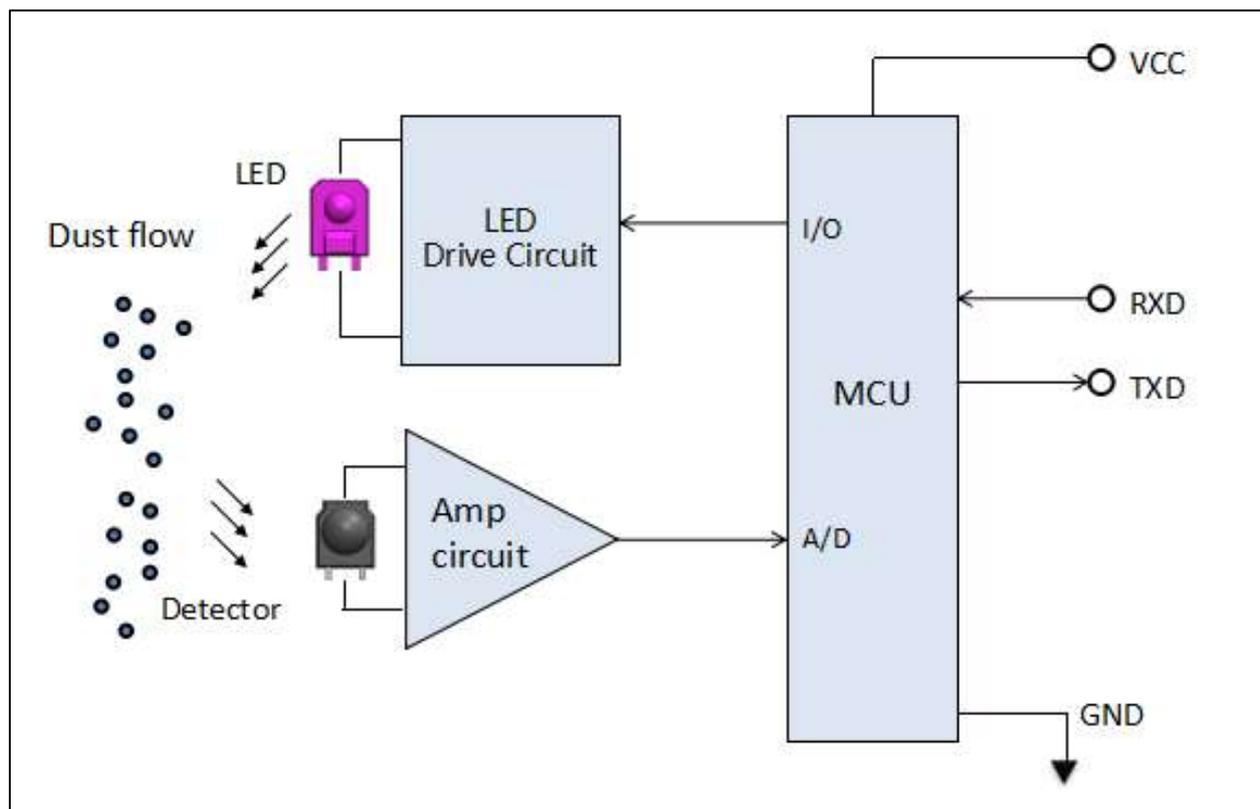
**Fig 1** Internal architecture
